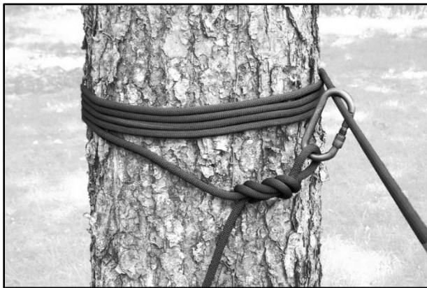
Figure 9-4. Example of tensionless, natural anchor
