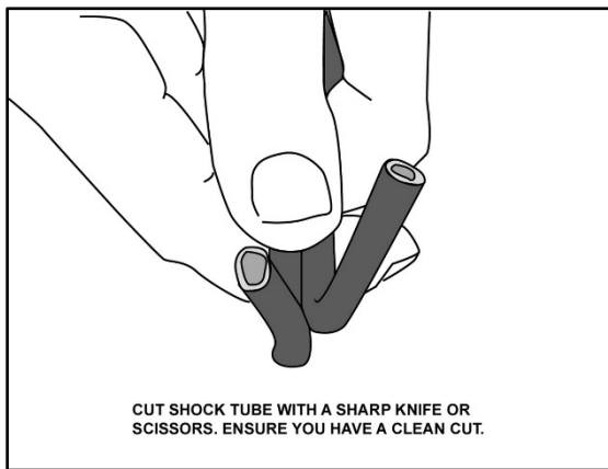
Figure 5-1. Technique for cutting shock tube
